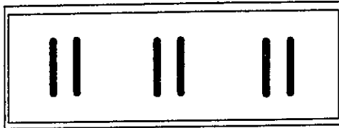
Figure 1 - Non-Segregated Phase Bus Cross Section
