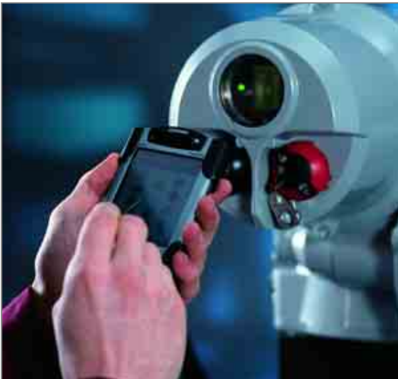
Below: Pocket IQ-Insight software tool used to download 'data logger' file.
