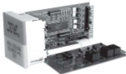
*Auxiliary Relay Module — Attached via ribbon cable to the Sequence Control Module*
