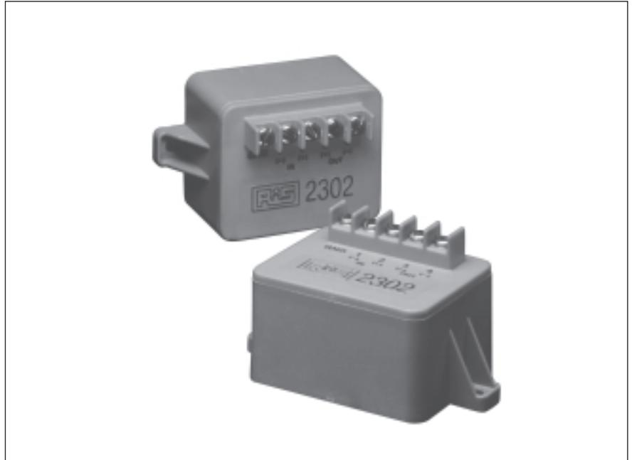
Ametek Loop Isolators are compact, low cost devices for isolating and converting common process current signals. They are loop powered from the input current, requiring no external power source.
