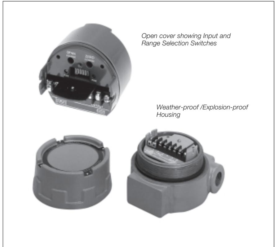
The Ametek Power Instruments Model SC-4372 2-Wire Transmitter accepts a Ni or Pt RTD input and generates a 4-20mA current output. The output is isolated and linearized to input temperature. The input type is single-jumper selected, and range is switch selected. One model of the SC-4372 covers both RTD types, 2 and 3 wire inputs, with full zero and span adjustability over the entire specified input range.
