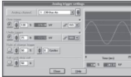
Analog Trigger Settings Window, where the Real Time Values for each Voltage and Current Input can be read.
