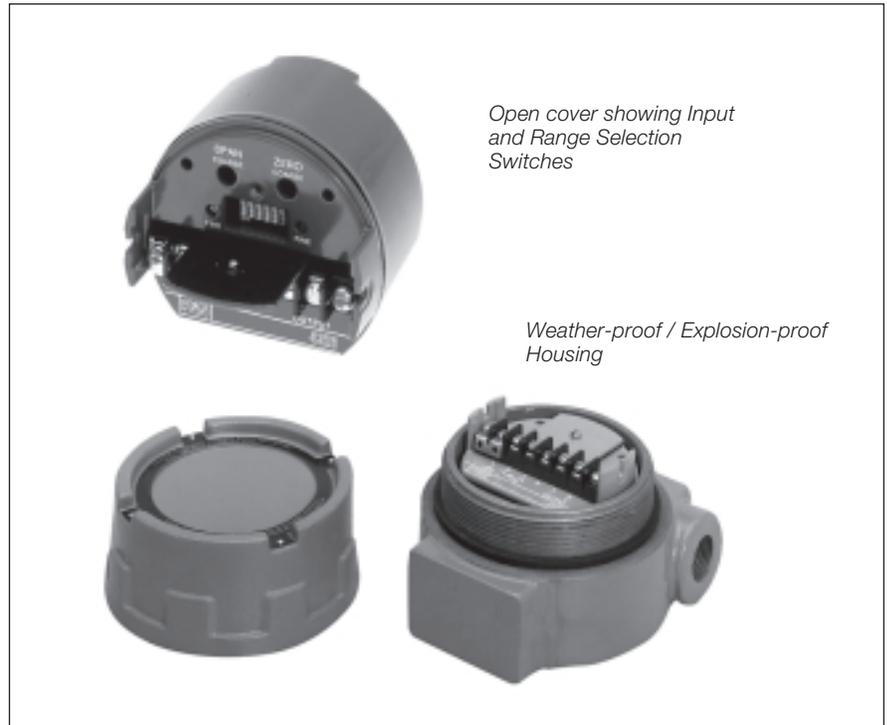
The Ametek Power Instruments Model SC-4300R 2-wire Transmitter accepts a slidewire input, typically from a position measurement device, and provides an output loop current of 4-20 mA proportional to the input resistance. The input may be anywhere in the range of 50 to 20K ohms. Span and zero offset adjustments are made with 16 position switches for coarse settings, and 25 turn potentiometers for fine adjustments. There are no components or jumpers to change in selecting the range.
