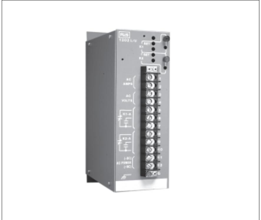
These single and dual trip alarms accept AC current or voltage inputs (field alterable) and provide one DPDT 5 amp (ET-1200L/U or two SPDT 5 amp (ET-1202L/U) universal relay contact outputs. Basic input spans are 16 to 200 VAC or 0-1 to 0-7.5 amps.
