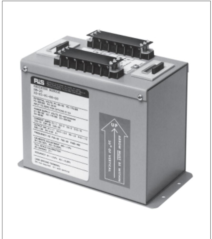
The Ametek Power Instruments watt-hour and VAR-hour register modules are an optional companion product to the Ametek watt/watthour (WWH) and VAR/VARhour (VVH) transducers. The RM-10 single register module will accumulate and visually display the total watthour or VARhour pulses from the WWH or VVH electronic transducers.
