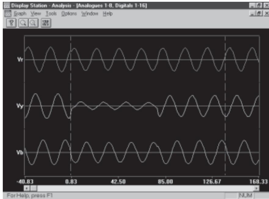
Waveform Capture (simultaneous on up to 16 analog and 32 digital inputs)
