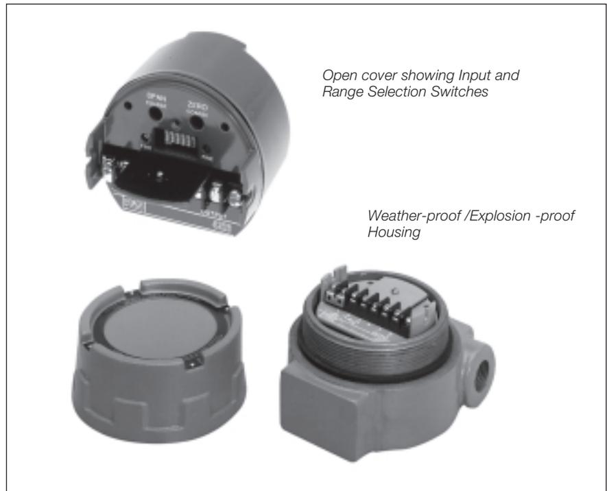
The Ametek Power Instruments Model SC-4326 2-wire Transmitter accepts a millivolt input from any specified thermocouple or millivolt source. The output is an analog 4-20mA current signal proportional to the millivolt input. The input type and range can be changed with switch settings on the transmitter, eliminating the need for jumpers or range resistors.
