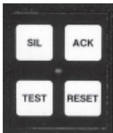
Pushbutton Control Module — with switch pad and power on LED
