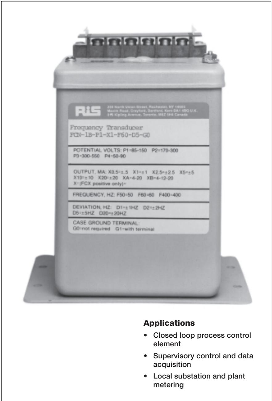
Ametek Power Instruments FCX and FCN Frequency Transducers are precision-engineered instruments designed to provide a constant current output into a variable impedance. The DC output from the device(s) very accurately represents the input frequency deviation from a selected center frequency of 50 or 60 Hz.
