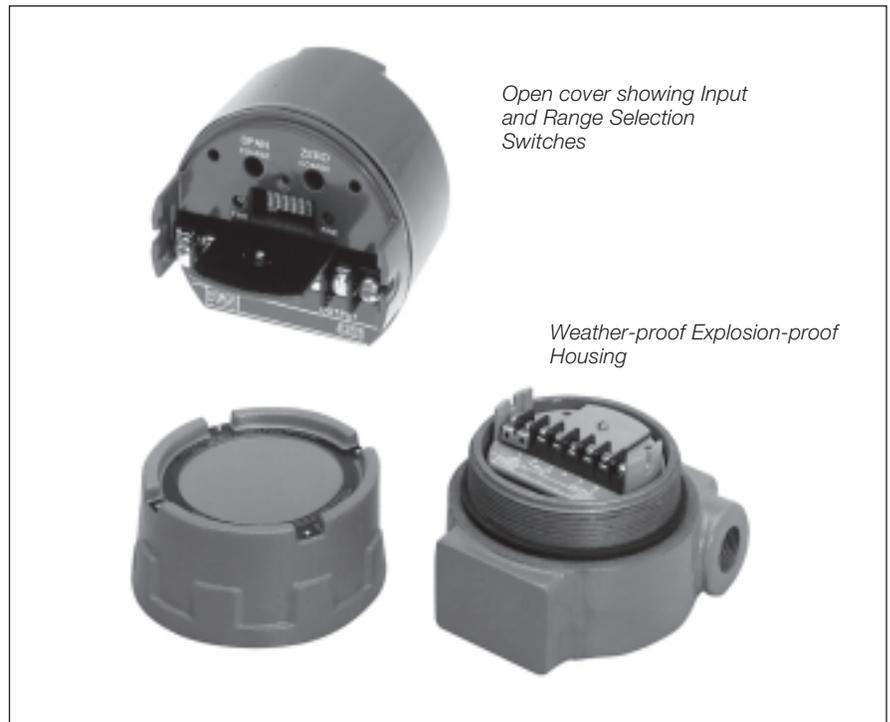
The Ametek Power Instruments model SC-4300 L/U is a 2-wire input selectable AC voltage or current transmitter. Both the input type and range are field selectable using easily accessible switches. The isolated 4-20mA loop current output is proportional to the input current or voltage with zero and span adjustability.
