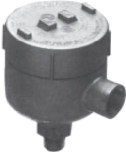
The Ametek Model VT-3360 Vibration Transmitter is a totally solid-state device providing vibration monitoring for non-critical rotating machinery. It combines a vibration sensor and electronics that provide for input power, 4-20 mA analog vibration output signal, and 0-1.0 mA vibration wave form output signal—all on just two wires. Various adjustments, sensing ranges and other features make the VT-3360 suitable for many vibration monitoring applications.
