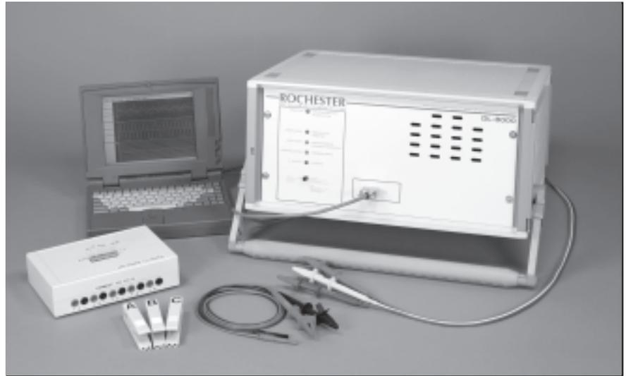
The DL-8000 and DL-9000 portables have been designed to be easily installed on-site, vastly reducing any commissioning time. The system includes optional push-fit (shrouded) protective rear panel connections to analog and digital measurement points using fused jaw-clips, pigtail leads and non-invasive CT clamps.
