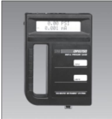
DPG-700 digital pressure gauges are hand-held calibrators that simultaneously display and measure pressure, vacuum and DC milliamp industrial process signals. They are battery powered and housed in rugged cases with membrane keypads to resist harsh industrial environments.
