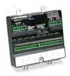
**EQ3720RM Relay Module** (Spec Sheet: 90-1181) The 8 Channel Relay Module is specially designed to expand the output capability of the Det-Tronics Eagle Quantum Premier System. The Relay Module provides eight channels of relay output points that are programmed for unsupervised operation. The output relays are rated up to 2 amps per channel at 30 Vdc maximum or 0.5 amps per channel at 120 Vac.
