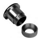
**Direct Duct Mount Assembly** (Spec Sheet: 90-1046). For mounting combustible sensors to air handling duct work. The Direct Duct Mount CGS assembly enables combustible gas detection in air handling, heating, ventilating, and air conditioning ducts. Designed for flat surface mounting only.
