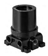
**EQ2200DCU Series Digital Communication Unit** (Spec Sheet: 90-1118) is approved for use with a variety of Det-Tronics sensors including PointWatch IR gas detector and hydrogen sulfide (H2S) electrochemical sensor (C706x Series). It will also accept any sensor/transmitter with a linear 4-20 mA output signal and allows for one person non-intrusive calibration. The DCU digitizes the analog signal and transmits the value to the controller.
