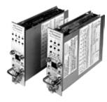
**R6006 Rack Mount Relay Output Module** (Spec Sheet: 90-1016). Units have eight individual form C relay outputs rated at 3 amps per relay. Relays can be operated by solid state outputs from one R7404, R7409 or R7494 controller. Zone relays can be grouped for voting outputs. R6006C and R6006D have load monitoring capabilities. Operates on either 12 or 24 Vdc. Mounts on Q4004 Cage Assembly (sold separately).
