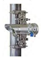
The **Open Path Eclipse Infrared Gas Detection System** (Spec Sheet: 90-1159) is a stainless steel, IR beam-type hydrocarbon gas detection system. The system consists of two modules (transmitter and receiver) offering:
