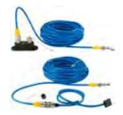
The **Remote HART Port Kit and Remote HART cable kit** (Manual: 95-8553) are used with the Model PIRECL PointWatch Eclipse IR gas detector to provide access to the Eclipse's optional onboard, intrinsically-safe HART port for a distance up to 20 meters. Cable set is 20 meter long, 2-core, shielded 20 awg conductors with overall PVC-jacket, and is IEC332 approved.
