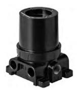
**EQ2200DCUEX Series Digital Communication Unit** (Spec Sheet: 90-1118) is a digital communication unit for catalytic combustible gas sensors (CGS). The DCUEX digitizes the analog signal and transmits the value to the controller.
