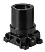
**EQ2500ARM Series Agent Release Module** (Spec Sheet: 90-1128) provides agent release capability for the Eagle Quantum System. The ARM is located on the LON and is controlled by programmable logic in the Eagle Quantum Premier Controller. The ARM can be programmed for "Single," "Cross" or "Counting" Zone Style initiation. Optional time delay, abort, and manual release sequences allow the output to be programmed for use in unique applications. Provides local control of releasing solenoids.
