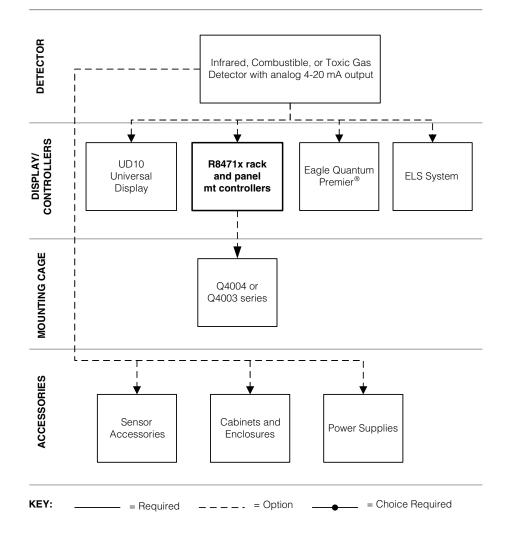
R8471 Single Channel Rack-Mounted Gas Controllers for use with Q4004 mounting cages (4U height)
