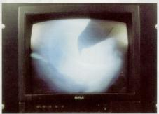
"The camera Plant personnel in the control room can watch coal igniting at the tip of the feed pipe inside the kiln on a monitor like this one. Corrective measures can from the pipe, be taken if workers spot problems.
